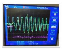
Figure 4b.CH2 O<u>utput/</u>₽ voltage of the inverter, CH3 <u>Grid</u> pulse₄input TWT, CH4 inverter current) Formatted: Caption
